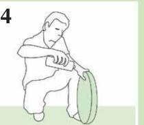
Use glue or duct tape to secure the circular pieces of ISOTHERM to the geyser.
