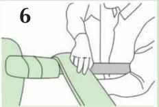
Use off cuts or cut a strips of ISOTHERM and wrap it around the pipes. Secure with duct tape.
