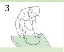
Cut out circles of ISOTHERM to be placed on the front and back of the geyser.
